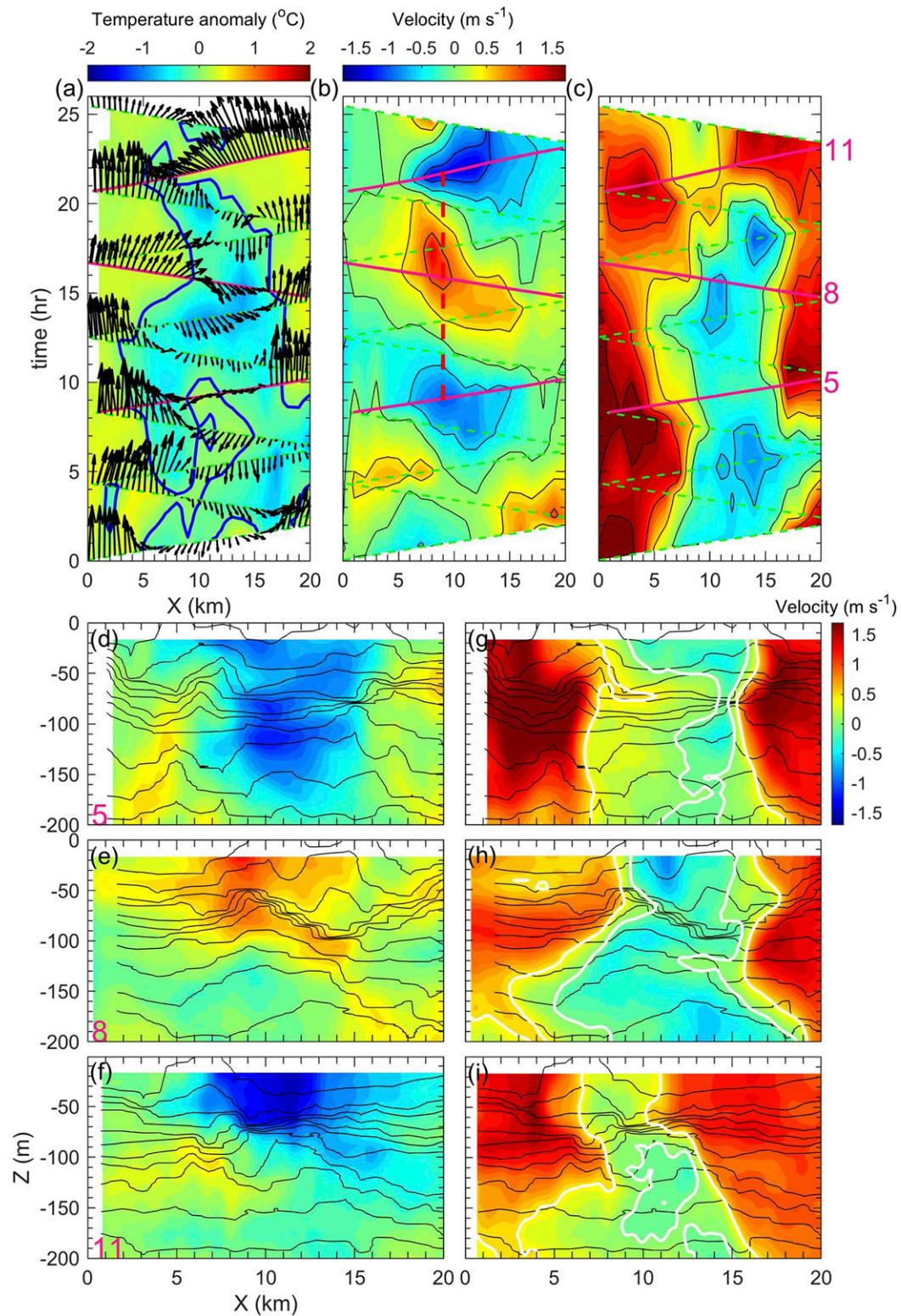
FIG. 7. Cross-wake distance–time contours of (a) temperature anomalies with corresponding current, (b) cross-stream, and (c) along-stream velocities measured at 20 m. Distance–depth contours of cross-stream velocity taken from surveys (d) 5, (e) 8, and (f) 11 and of along-stream velocity taken from surveys (g) 5, (h) 8, and (i) 11. The magenta lines shown in (a)–(c) show patterns identified from surveys 5, 8, and 11 overlain on
