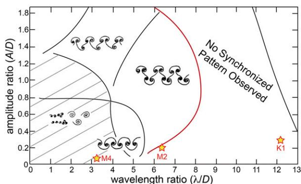
FIG. 11. Synchronization and vortex patterns based on  $\lambda/D$ – $A/D$  diagrams reproduced from Williamson and Roshko (1988). The black curves depict different wake pattern regimes. The red curve separates the diagram into nonsynchronization and synchronization regimes. The stars show the positioning of the  $K_1$ ,  $M_2$ , and  $M_4$  tides.
