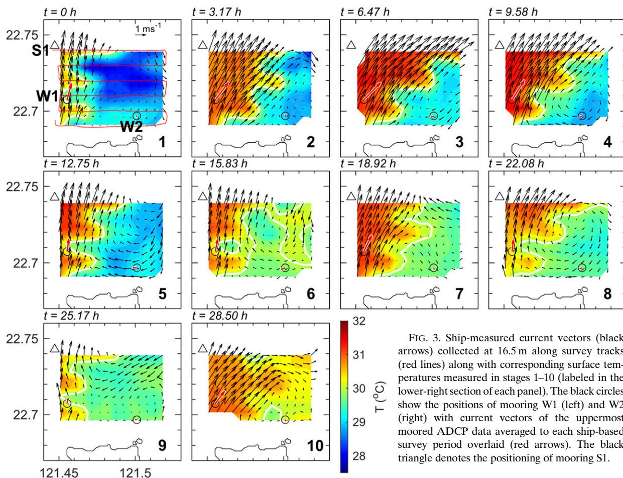
FIG. 3. Ship-measured current vectors (black arrows) collected at 16.5 m along survey tracks (red lines) along with corresponding surface temperatures measured in stages 1–10 (labeled in the lower-right section of each panel). The black circles show the positions of mooring W1 (left) and W2 (right) with current vectors of the uppermost moored ADCP data averaged to each ship-based survey period overlaid (red arrows). The black triangle denotes the positioning of mooring S1.
